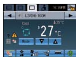
GROUP screen Displays the detailed operation status of each group. Sets group operations.
